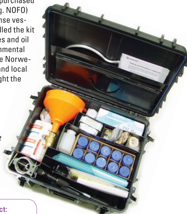
Fig.1. The new oil spill sampling kit developed by SINTEF
