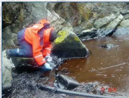
Scientist Janne L. M Resby from SINTEF taking samples of stranded emulsified heavy fuel oil
